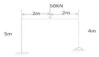
Q3. Analyse the rigid frame shown in Fig. by moment-distribution method. The moment of inertia of all the members is shown in the figure. Neglect axial deformations.
