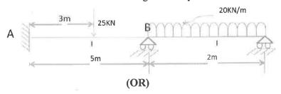
• Q8. Using the stiffness method, analyze the beam shown in the figure below.
